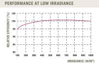
The typical change in module efficiency at an irradiance of 200 W/m<sup>2</sup> in relation to 1000 W/m<sup>2</sup> (both at 25 °C and AM 1.5 G spectrum) is -1.5% (relative).
